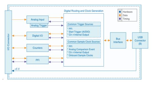
Fig. 1. National instruments - DAQ 6210 block diagram
