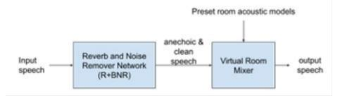
Figure 2: Block Diagram of Two-Stage Virtual Acoustic Background System
