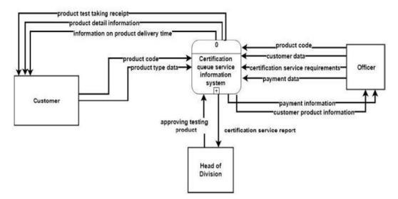
Fig. 4 Context diagram on priority service for certification queue service information system
