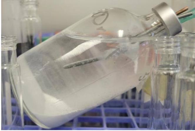
Figure 2) Serum bottle laid on test tube rack to allow ZnO NPs to precipitate for easier extraction.
