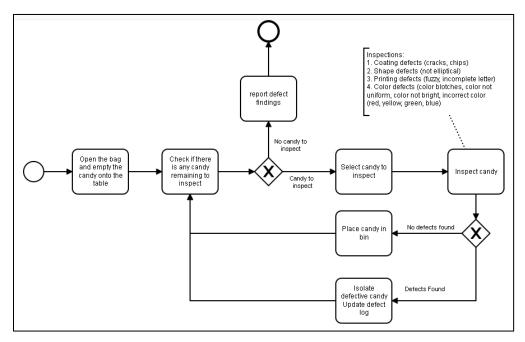
Figure 1. Sample Inspection BPMN Diagram
