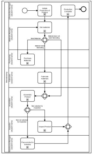
Figure 5. Sample High-Level Product Manufacturing BPMN Diagram
