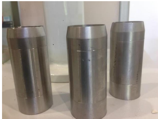
Figure 3.8: Standard mould for UCS test
