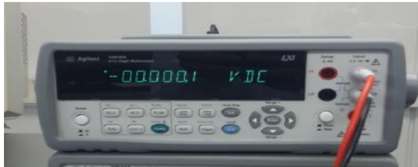
Figure 12: DMM used for testing connectivity and resistance measurements
