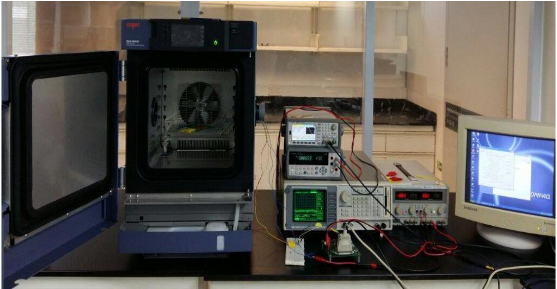
Figure 17: The connection of the humidity sensor to the laboratory equipment
