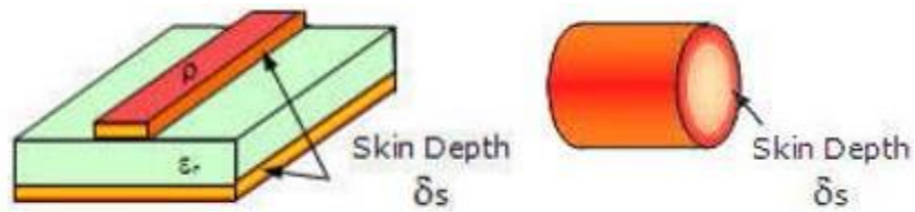
Figure 2. 6: Skin depth of a conductor [29]
