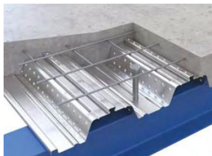
FIGURE 7 Composite Slab (Tata Steel Europe, n.d.)
