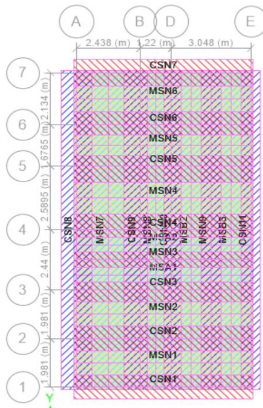
FIGURE 5 Design Strips Modelled on Raft Foundation
