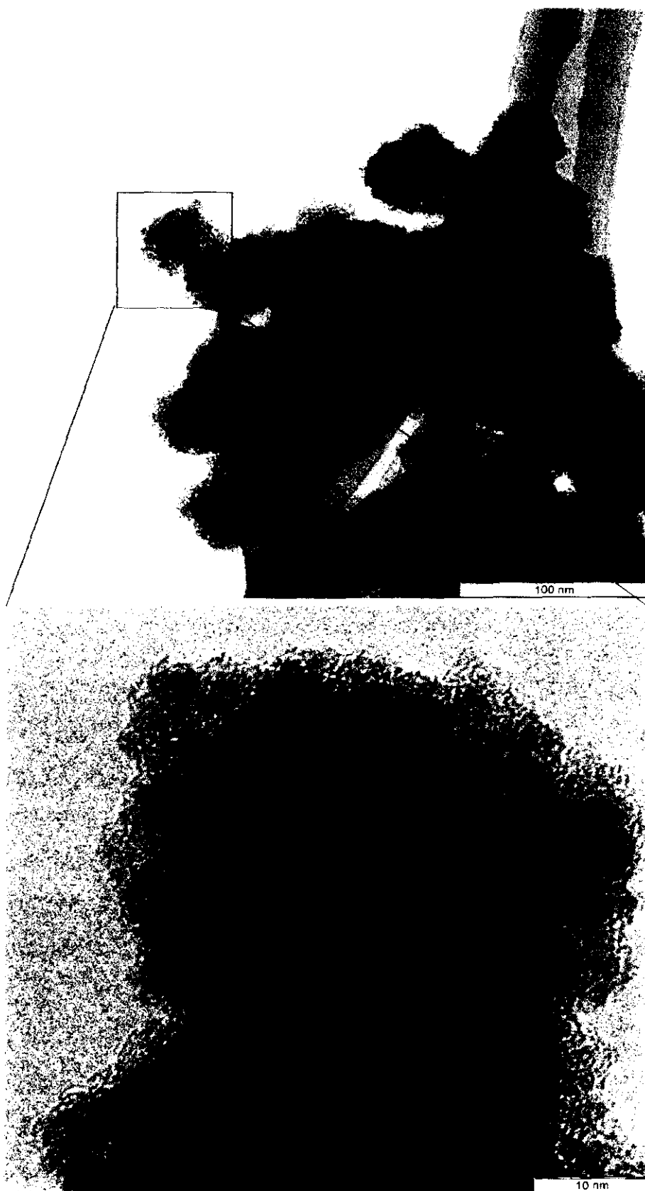
Figure 4.15: TEM images of iridium oxide electrodeposited by cyclic voltammetry
