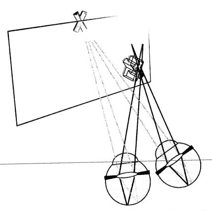
Figure 2.3: Accommodation – vergence response in stereoscopic 3D TV. Green 'X' is placed behind the screen and the eyes focus on the screen but the object appears at the back. This is called negative or uncrossed disparity. In the case of positive or crossed disparity, the object appears in front of the screen and the eyes are focused on the screen through cross viewing. When depth changes, there is a conflict in accommodation and vergence responses of the visual system.
