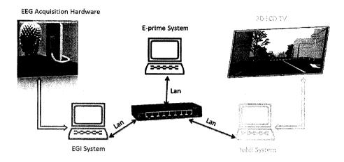
Figure 3.5: Hardware configuration of the three systems using a network adaptor through ethernet cables.
