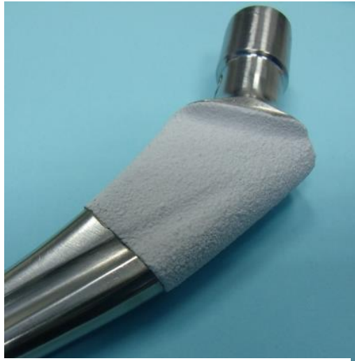
Figure 2.5 Partially HA coating on metal implant
