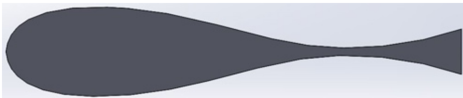
Figure 3-2: 20cm length, 10cm trailing edge (Top view)
