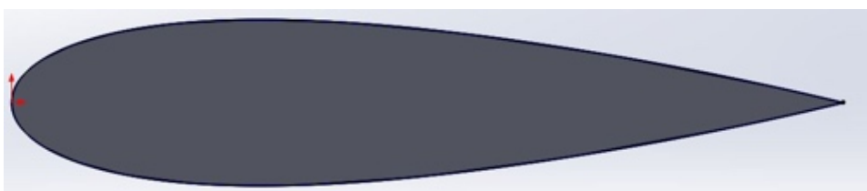
Figure 3-4: NACA 0020 (Top view)
