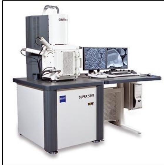
Field Emission Scanning Electron Microscope (FESEM).
