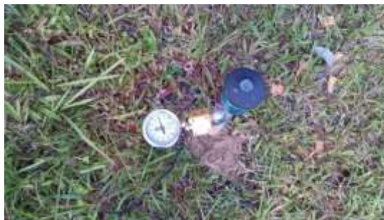
Figure 3.3: Pressure transducer fitted at individual tensiometer.
