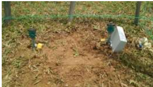
Figure 3.2: Two tensiometer were installed in different depths.
