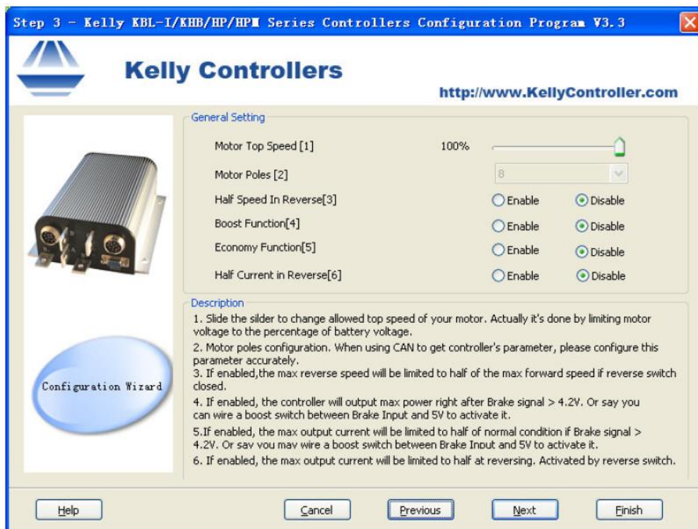
Figure 38: Kelly Controller setting step 3 [21]
