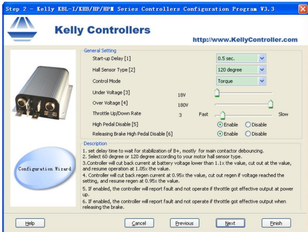
Figure 37: Kelly Controller setting step 2 [21]
