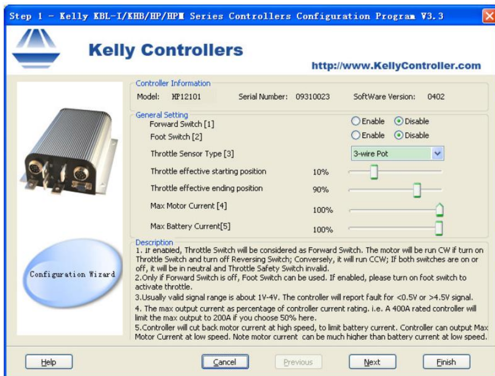
Figure 36: Kelly Controller setting step 1 [21]
