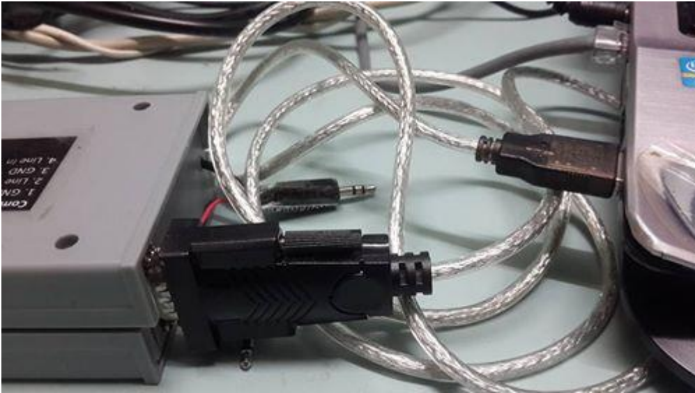
FIGURE 3.11. Com port connection (RS 232)
