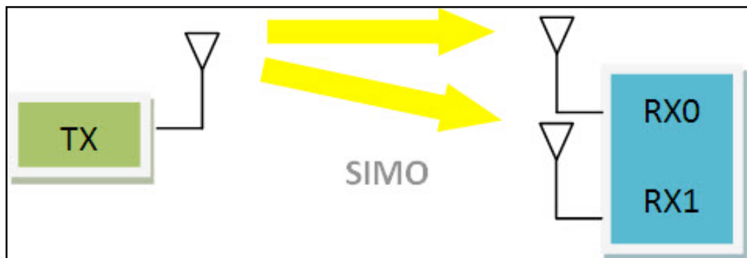
FIGURE 1.1. The Transmission Mode of SIMO (single input multiple output)
