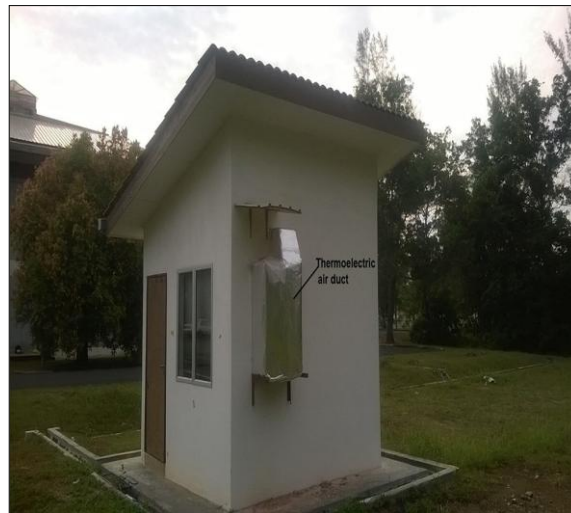
Figure 3.4. Test room equipped with TE-AD [26]
