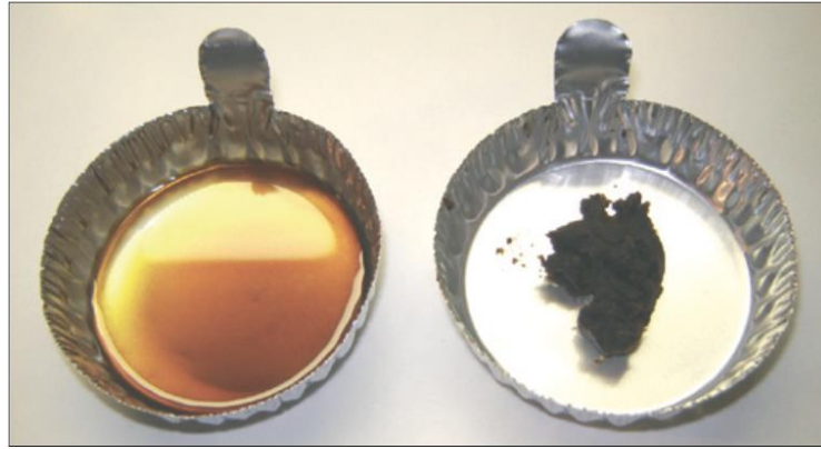
Figure 11: Crude oil sample above WAT (left) and crude oil sample below WAT (right) (The figure obtained from PerkinElmer to show the possible outcome after using DSC)[24].
