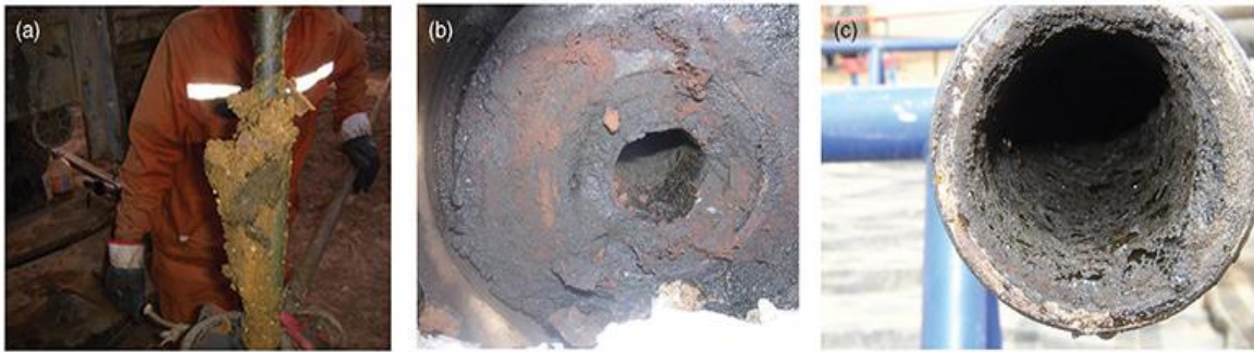
Figure 2: The effect of wax deposition is shown on (a) a well tubing string, (b) a cross-section of a flowline, and (c) the inside of a tubular [4]
