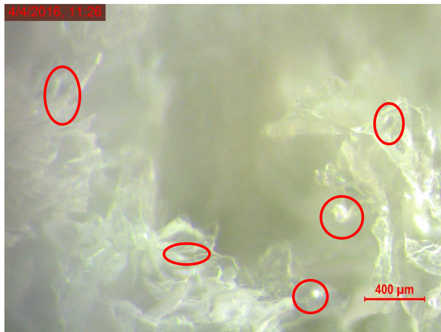
Figure 22: OM image for steel X65 Precipitated with 10% paraffin wax (x10 magnification) Red circle indicate kerosene drops.
