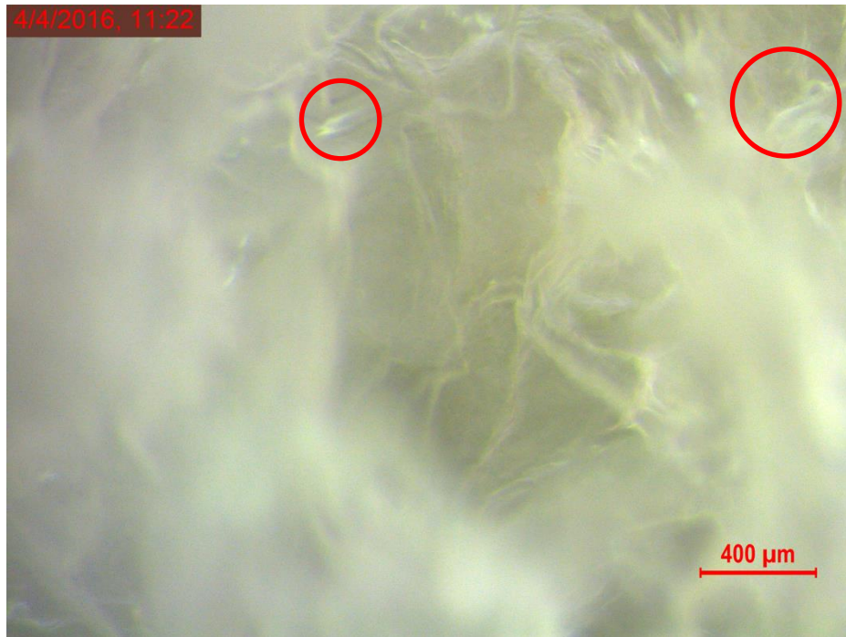
Figure 21: OM image for steel X65 Precipitated with 10% paraffin wax (x10 magnification) Red circle indicate kerosene drops.
