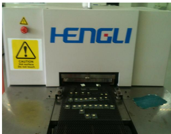
h. Photoelectrode sintered in oven after screen printing of titanium oxide
