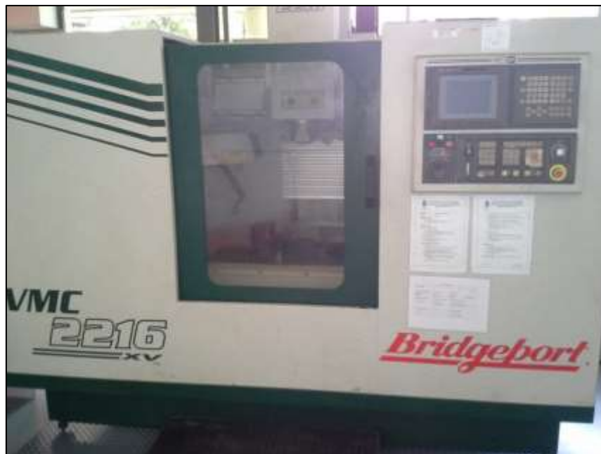
Figure 8 CNC Bridgeport Milling Machine used to imitate FSW Machine
