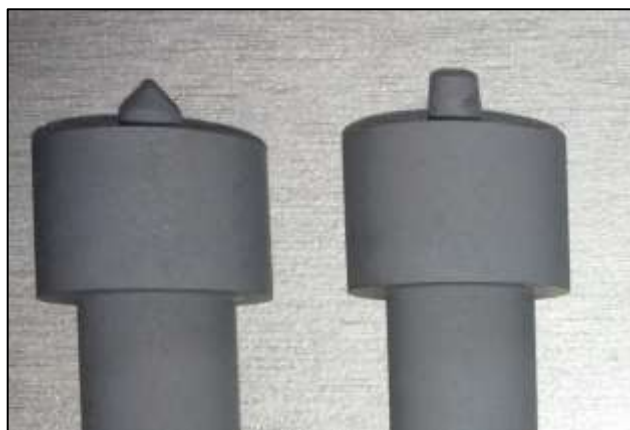
Figure 7 pin tool made from AISI D2 Tool Steel after heat treatment
