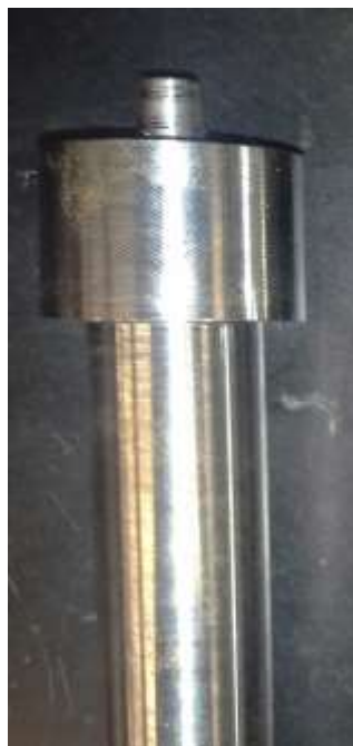
Figure 6 tapered pin tool made from H13 Tool Steel
