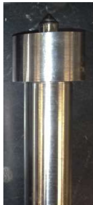
Figure 9 half-cone pin tool made from AISI D2 Tool Steel
