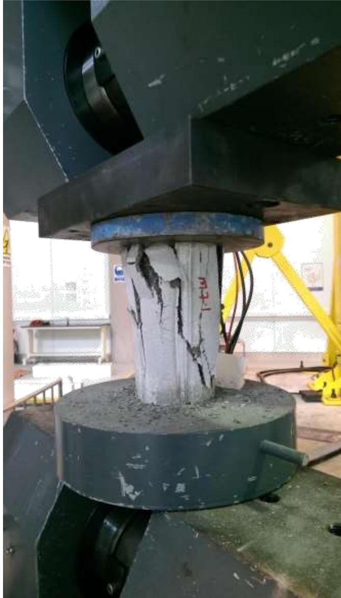
Figure 23: Samples Compression Test
