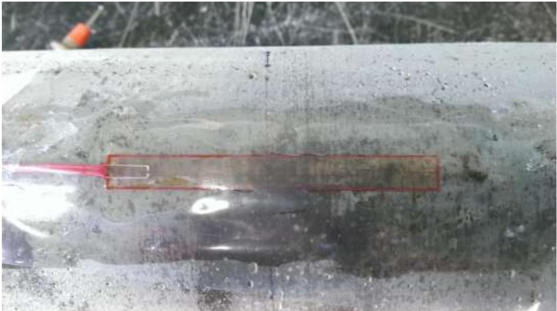
Figure 17: Strain Gauge installed on ECC sample
