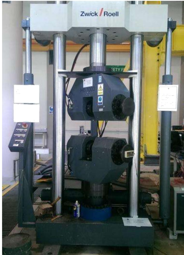
Figure 20: The equipment used to test sample stress-strain behavior
