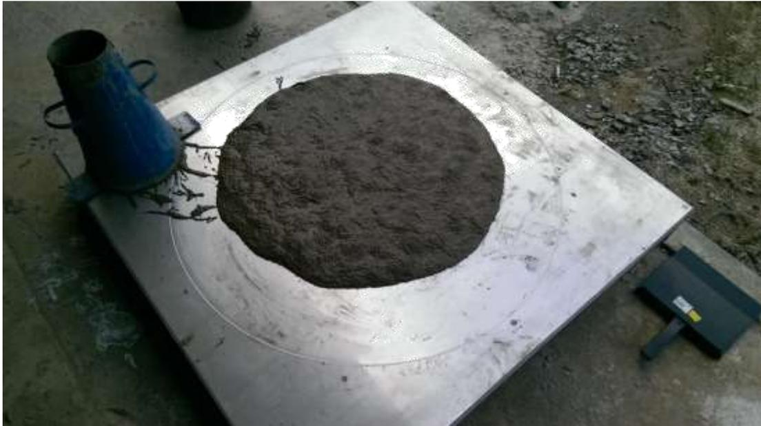
Figure 14: Flow table test to measure sample workability
