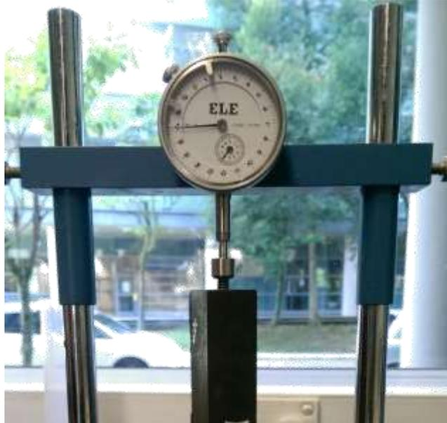
Figure 16: The comparator used to measure change in sample length
