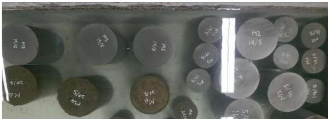
Figure 13: Samples molded are cured for 28 days before testing
