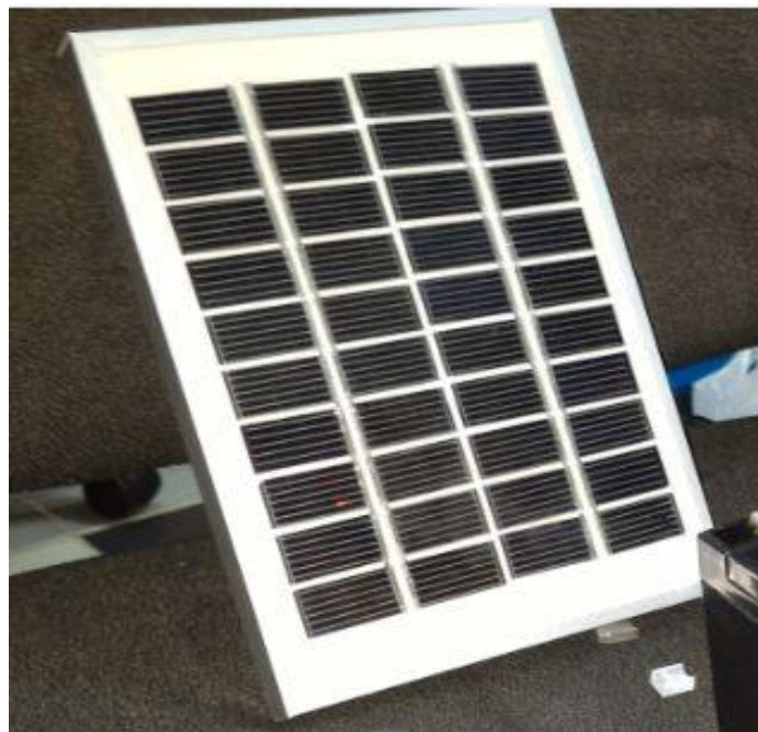
Figure 19: Solar Panel 6V 3A
