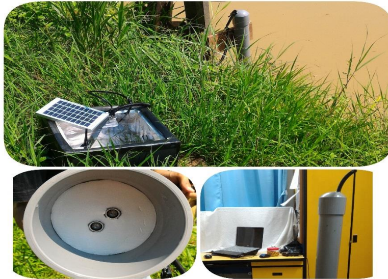
Figure 15: Ultrasonic installed in field testing
