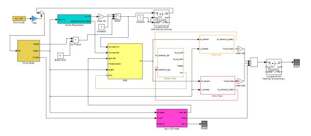
FIGURE 4.2: MATLAB/Simulink HEV model overview
