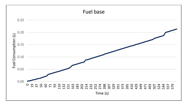
FIGURE 5.9: Fuel consumption for base vehicle model (NYCC)
