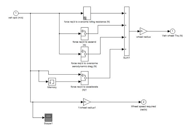
FIGURE 4.4: Vehicle requirement block model
