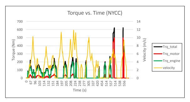
FIGURE 5.2: Torque distribution for HEV model (NYCC)
