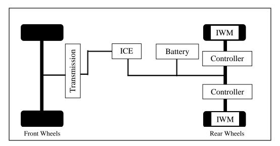
FIGURE 1.3: Parallel configuration of components in HEVs [10]
