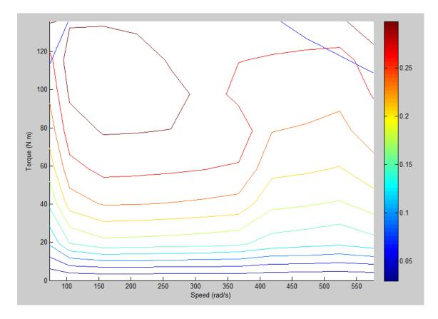
FIGURE 4.19: ICE efficiency
