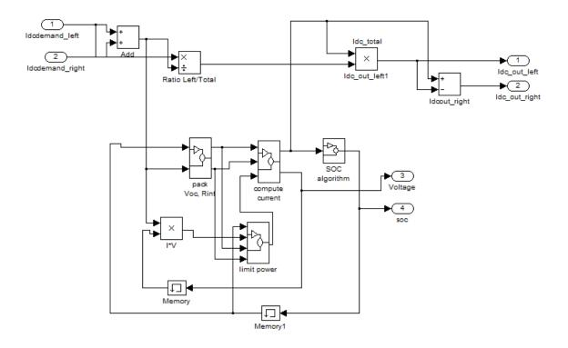
FIGURE 4.26: Battery pack model
