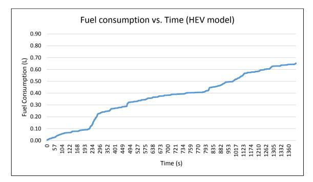
FIGURE 5.6: Fuel consumption for HEV model (UDDS)
