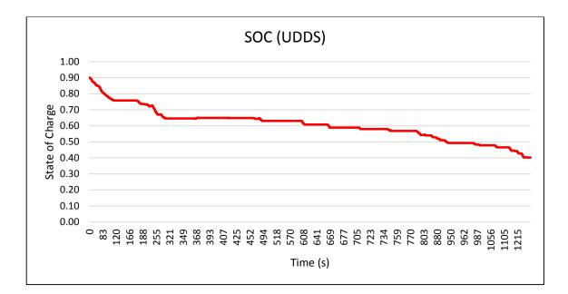
FIGURE 5.4: SOC in battery pack (UDDS)
