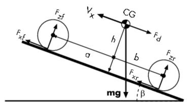
FIGURE 4.9: Vehicle dynamics and motion
