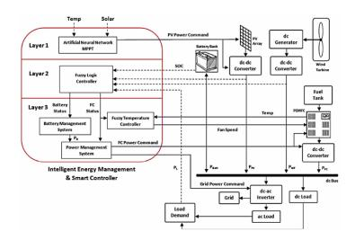
FIGURE 2.2: Block diagram of the proposed system [3]
