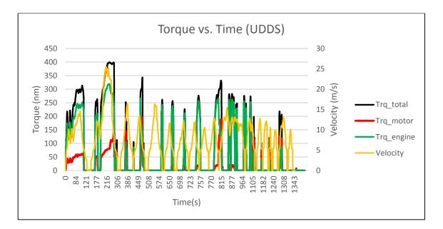
FIGURE 5.1: Torque distribution in HEV model (UDDS)
