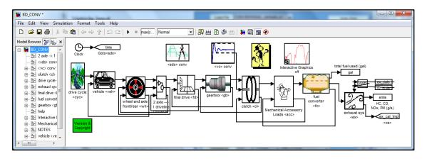
FIGURE 4.11: Vehicle model Block Diagram developed in ADVISOR
