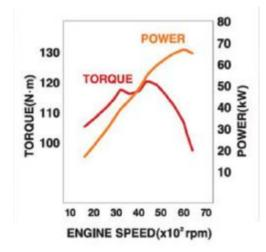
FIGURE 4.5: Graph of Torque and Power VS Engine Speed. [13]
