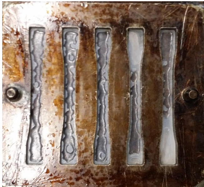
Figure 3-9 Dog-bone shape LDPE layers
