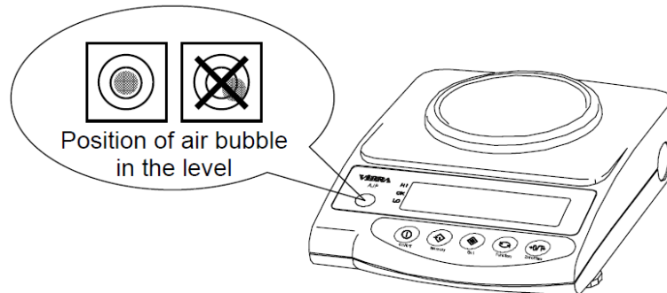
Figure 3.6: Securing the exact level of the balance
