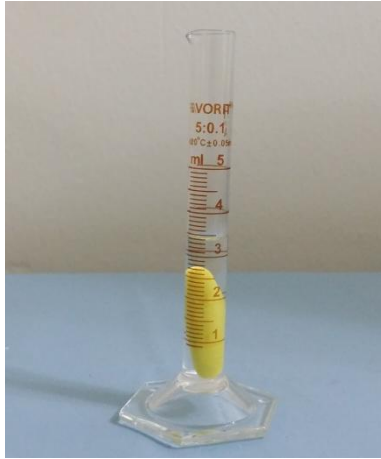
Figure 3.10: The mould material placed into the measuring cylinder which filled with 2ml distilled water
