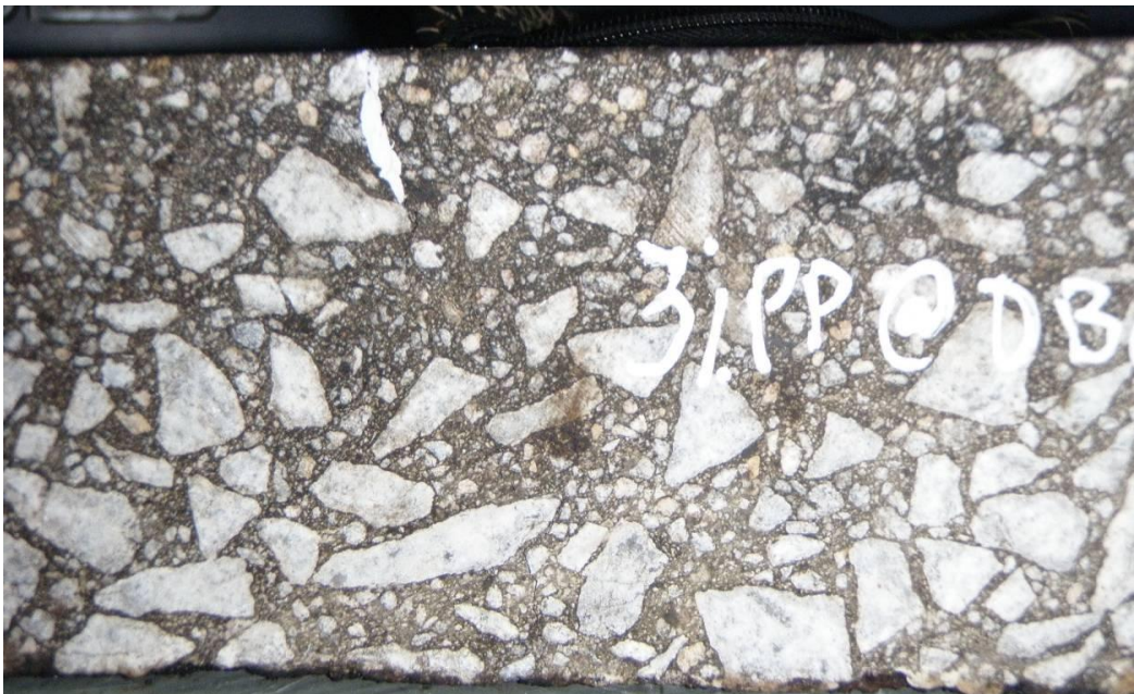
Figure 16: Crack Pattern observed for 3% PP PMB Bituminous mixture beam
