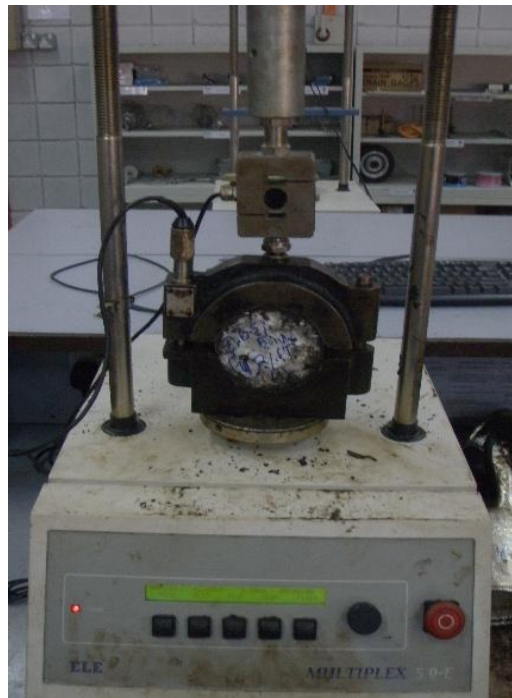
Figure 3.13: (a) Marshall Specimen (b) Marshall Testing Machine
