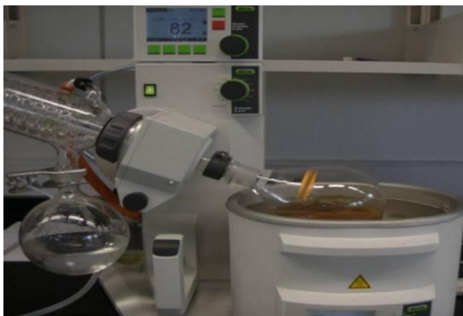
Figure 3.8: Removal of solvent using rotavapor
