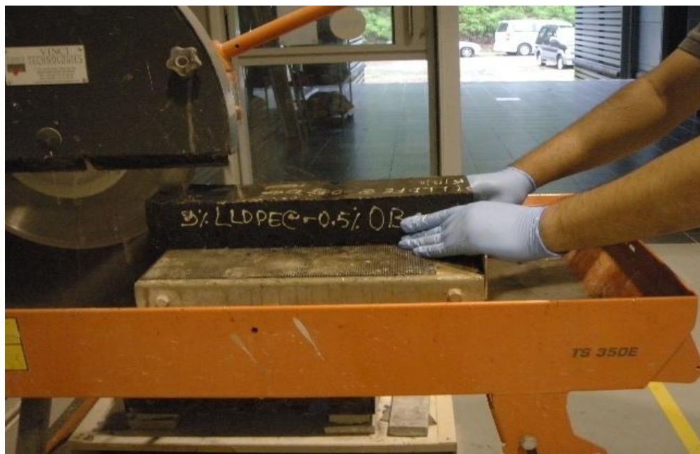
Figure 3.20: Saw cutter used for cutting of beams
