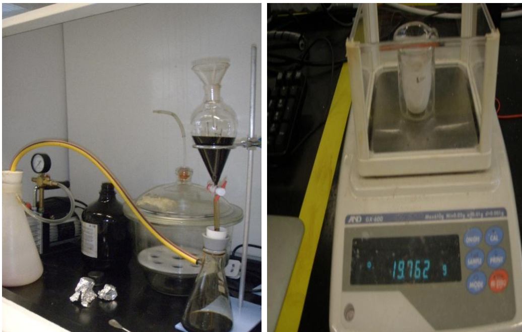
Figure 3.4: (a) Filtering n heptane solution (b) Weighing collected precipitated asphaltene on glass fibre filter pad
