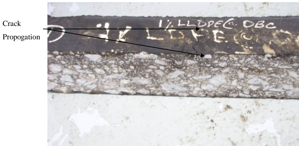
Figure 8.11: Fatigue crack pattern observed for LLDPE Specimen
