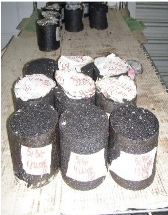
Figure 3.13: (a) Marshall Specimen (b) Marshall Testing Machine
