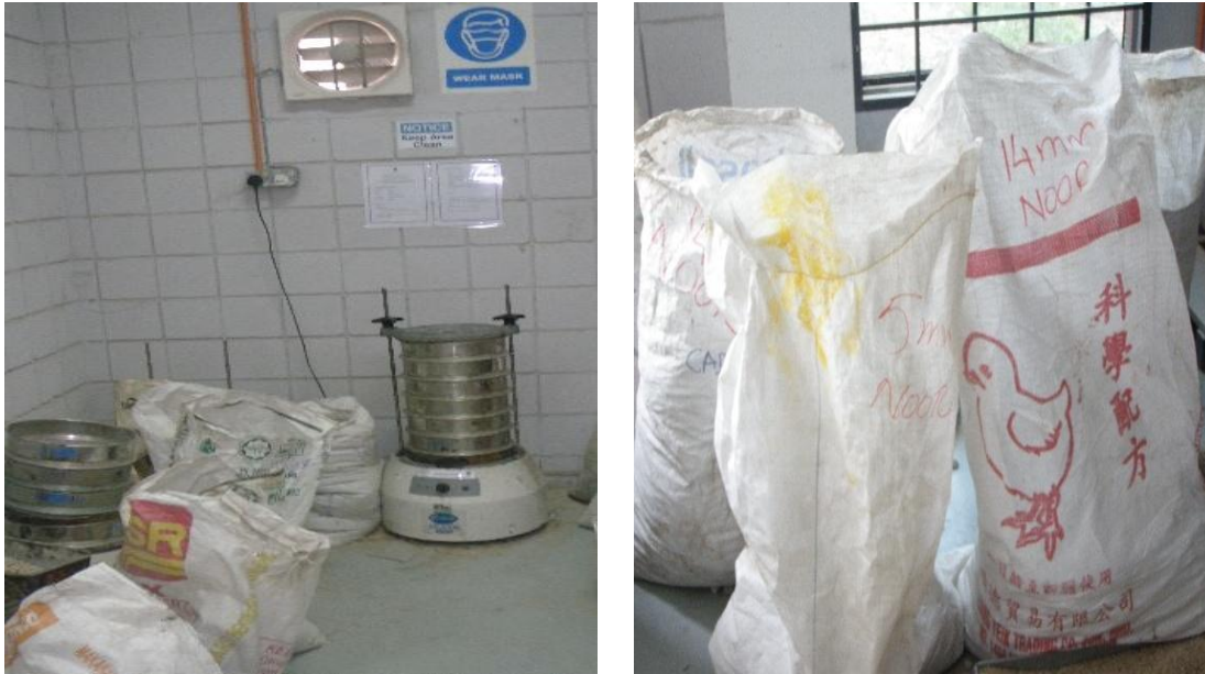
Figure 3.2: Sieve Shaker along with the bags for storing individual sieve sized aggregate
