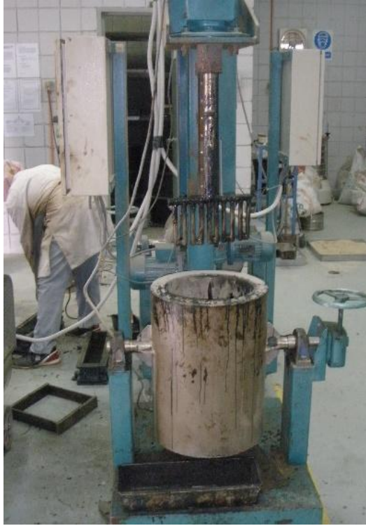
Figure 3.12: (a) Electric Mixer (b) Gyrotory Compactor
