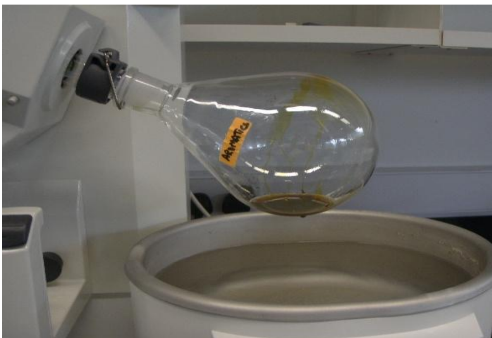
Figure 3.9: Left over bitumen fraction after solvent removal by rotavapor
