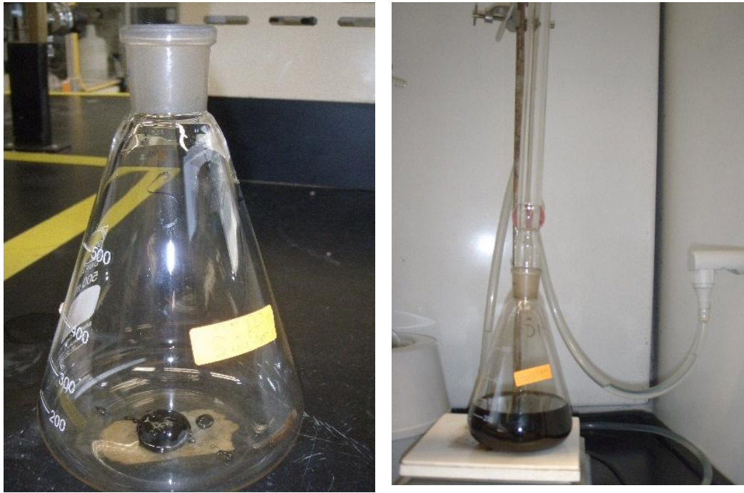
Figure 3.3: (a) Bitumen sample in Erlenmeyer flask (b) Erlenmeyer flask on hot plate with reflux condenser
