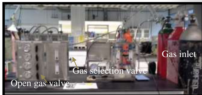
Figure 3-10: Gas permeability Unit at Block 3, UTP
