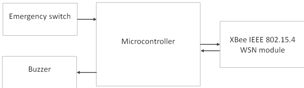
FIGURE 17: Block Diagram of Personnel Node
