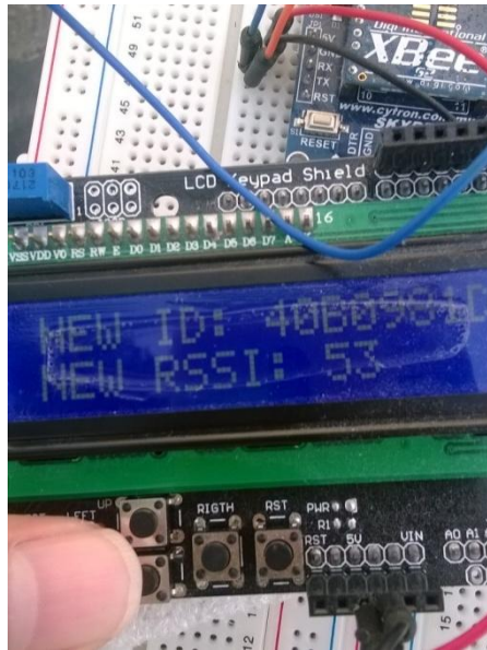
FIGURE 14: Extracting RSSI Value from WSN Module
