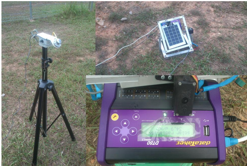
Figure 14: Pyranometer, PV panel and DataTaker
