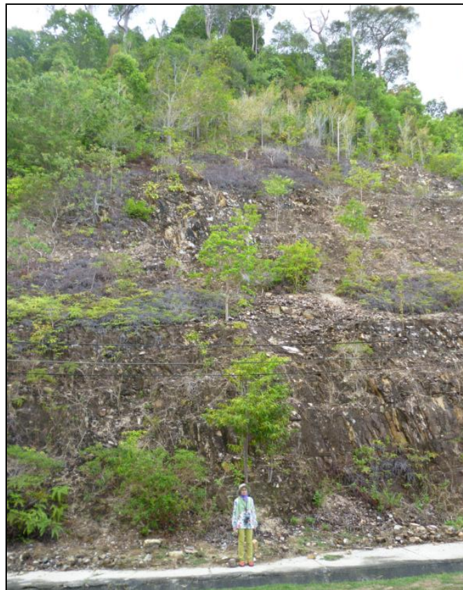
Figure 14: Outcrop 3 is weathered and fractured. The sandstone surface has been weathered by iron oxide giving brownish to orange colour. The top part of the outcrop was out of reach by the author due to HSE issue.
