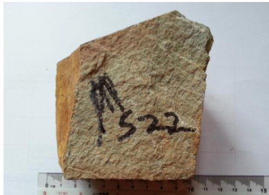
Figure 27: Sample 22. Very fine metaquartzite. Location: Outcrop 8.
