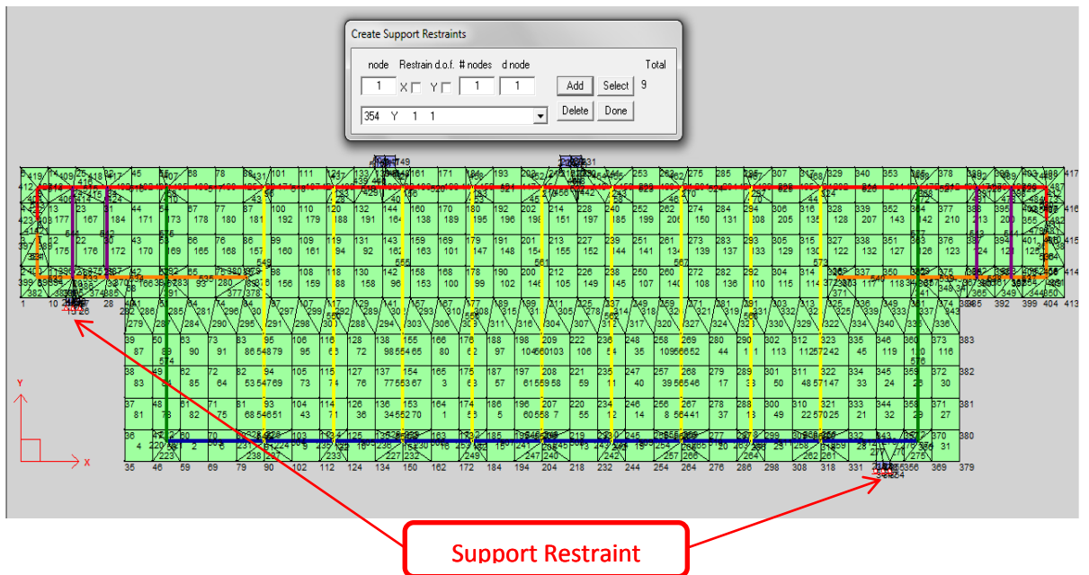
Figure 17: Creating Support Restraint
