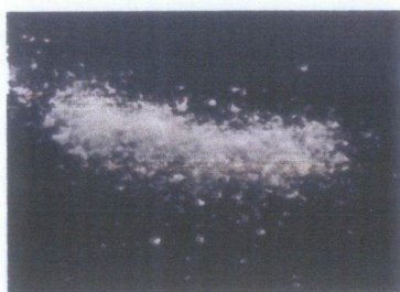
Figure 9: The CaCl 2 product from reacting HCl and cockle shell.
