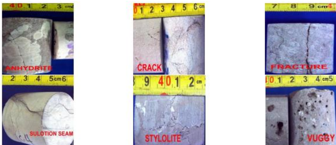
Figure 2.4: Geology phenomena on core in research area
