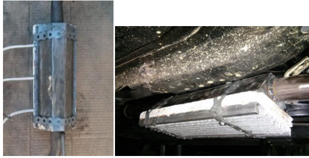
Figure 4.15: Installation of TEG on exhaust pipe
