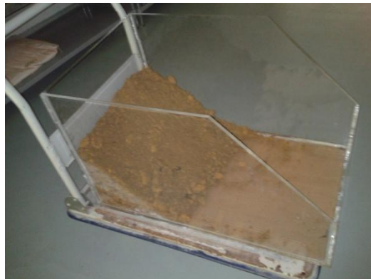
Figure 42: Perspex container with soil sample
