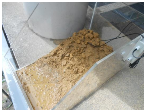
Figure 46: Sedimentation occur due to high porosity
