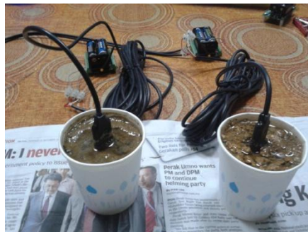
Figure 29: EC-5 moisture sensor immersed in soil sample
