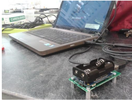
Figure 30: Base station for data acquisition connected to PC
