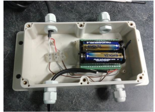
Figure 44: IRIS and MDA300 board is placed in waterproof container
