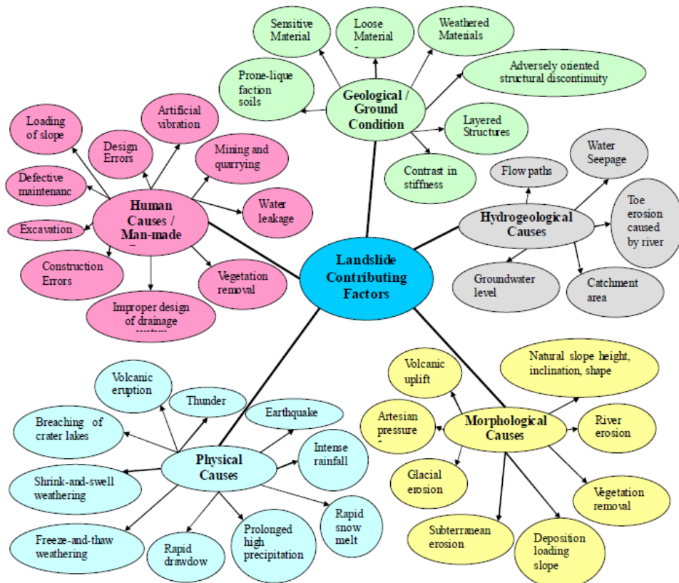
Figure 6: Landslide contributing factors[15]
