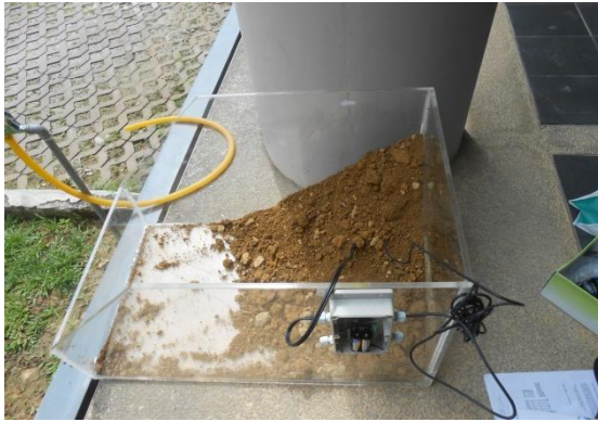
Figure 43: Sensors are plant at the middle of the slope
