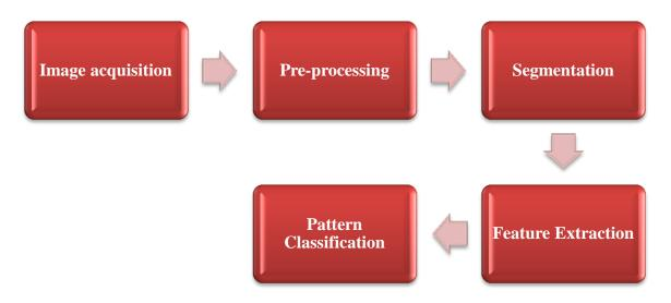
Figure 5: Image processing flow
