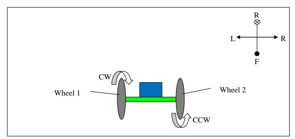
Figure 17: Illustration for Servo Motor Manoeuvre
