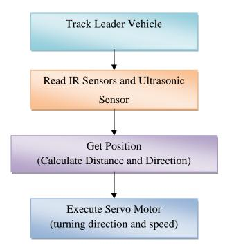
**Figure 7: Architecture of software**
