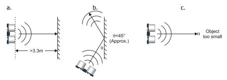
Figure 10: Factors affecting PING))) ultrasonic sensor [19]
