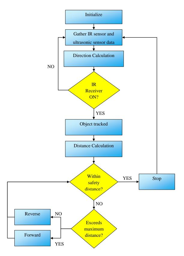
Figure 8: Object-tracking Algorithm
