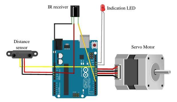
The figure below is the setup of connections. On the follower vehicle, the connections are as follow:
