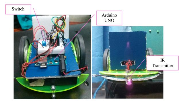
Figure 28: Front and Back View of Leader Vehicle
