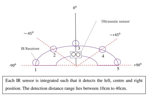
The sensors are arranged in this manner (arc form) in order to be able to tell which zone the targeted object is currently at. For example, if the IR 1 lights up that mean the targeted object is at position of far left most.
