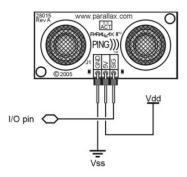
Figure 4: PING))) Ultrasonic Distance Sensor [19]
