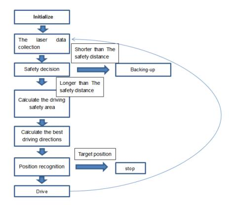
Figure 2: Autonomous driving systems [8]
