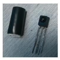
Appendix 2: Infrared Receiver with non-reflective sleeve
