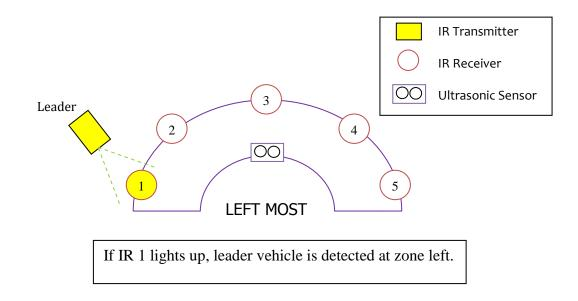
IR 1 and IR 2 detects left zone, IR 3 detects middle and IR 4 and IR 5 detects right zone.
