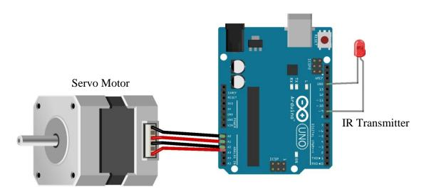
Figure 13: Connection of sensors and other components for leader vehicle
