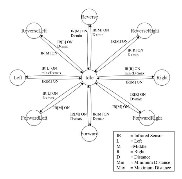
**Figure 9: Finite State Machine**
