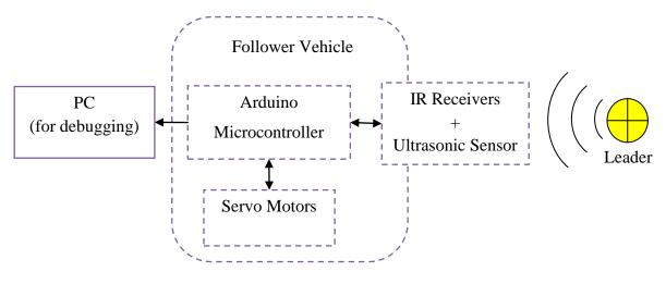
Figure 6: Architecture of object tracking system
