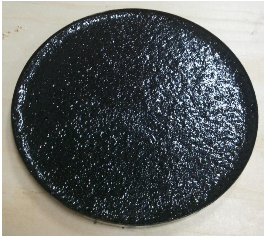
Figure 5.3: 10% Rice Husk bitumen's appearance (After Aging)
