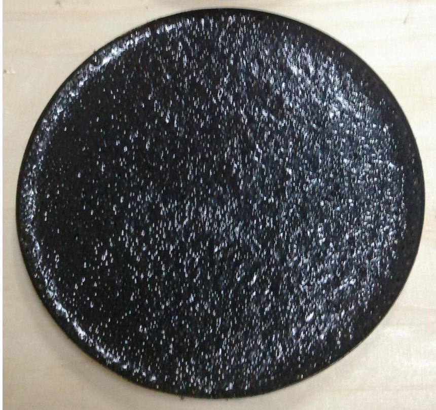
Figure 5.2: 5% Rice Husk bitumen's appearance (After Aging)
