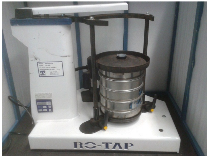
Figure 3.3: Testing sieve shaker and nest of U.S.A sieve pan
