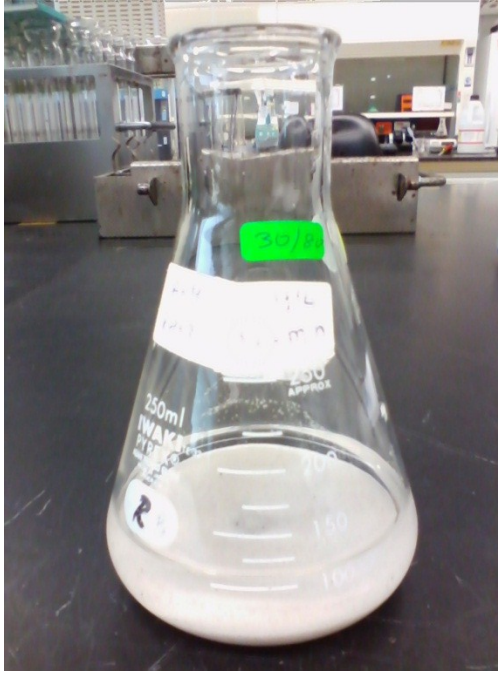
Figure 3.5: Mixture of sand sample and demineralized water in conical flask
