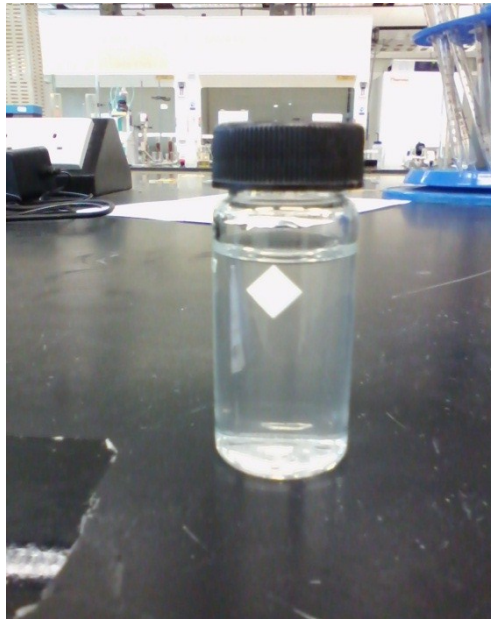
Figure 3.6: Test vial fill with the water-silt suspension
