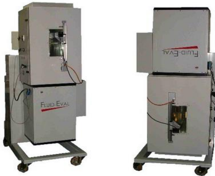
Figure 8: Fluid-Eval Standard Version which is used to measure bubble and dew points.
