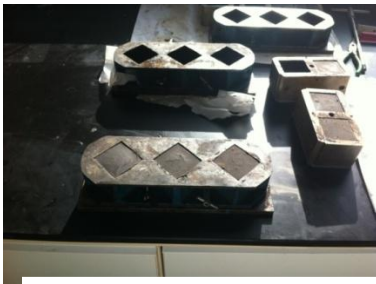
Figure 3.7 shows the geopolymer paste soon after mixing and nicely slotted into the cube moulds.
