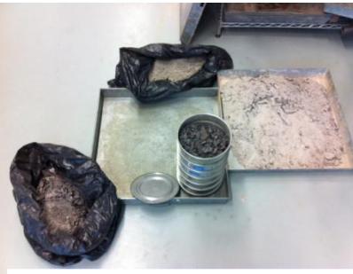
Figure 3.2 shows the remnants wood from the sieved fly ash in the sieving cylindrical pan and accumulated fine fly ash in the black plastic bag on the top.
