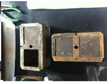
Figure 3.8 shows another mould ready to be cured in the oven for 24 hours.
