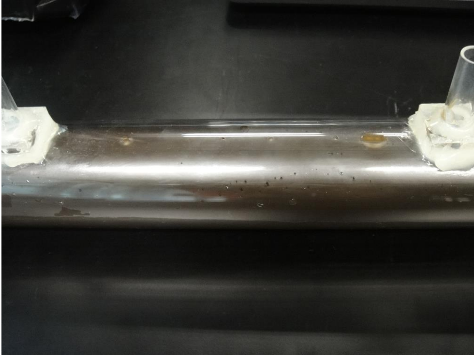
Figure 4.1: The image of voids formation before injecting air
