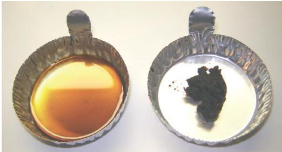
Figure 2.2: Crude oil sample above WAT (left) and Crude oil sample below WAT (right)
