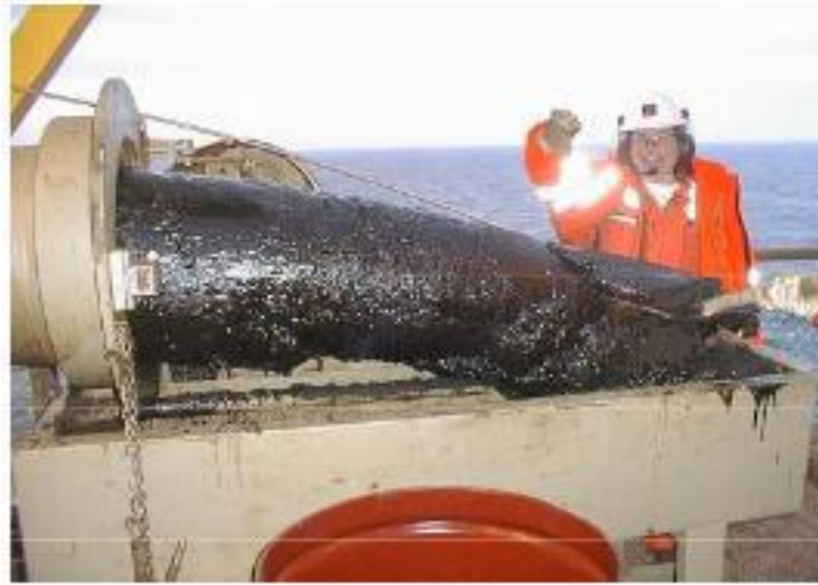
Figure 2.9: Gelled plug removed through pigging
