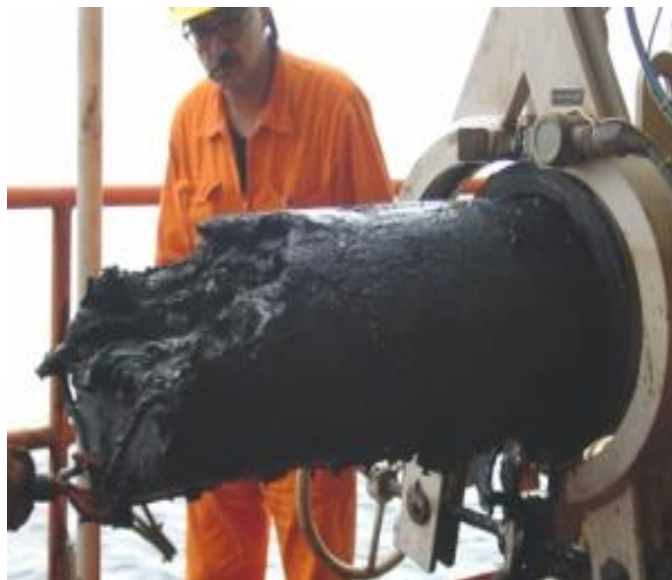
Figure 2.11: Critical gelled crude oil that stuck in pipeline in Gulf, Mexico
