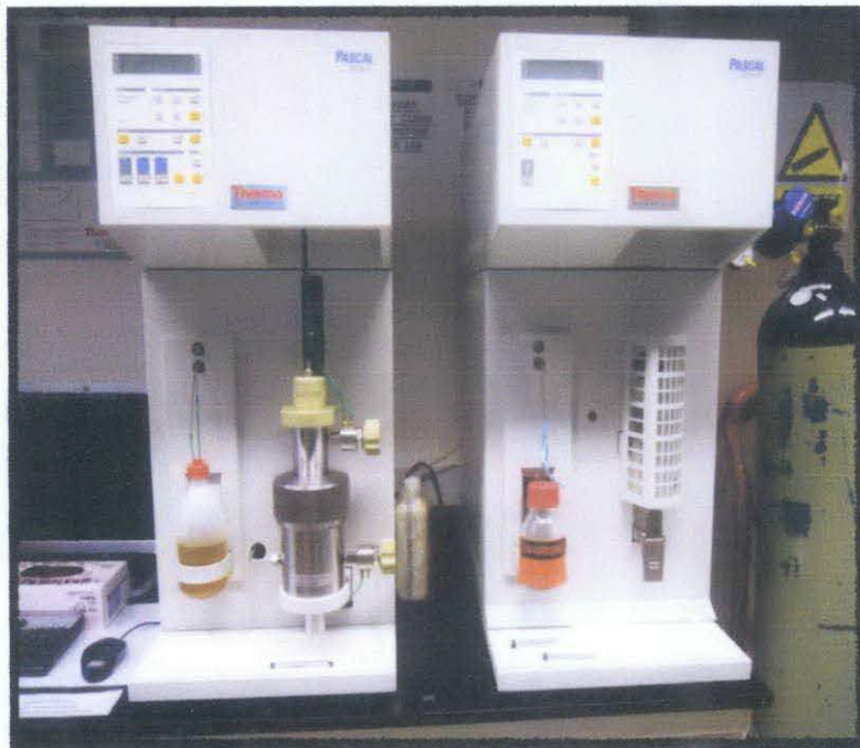
Figure 3B Porosimeter to determine porosity and permeability
