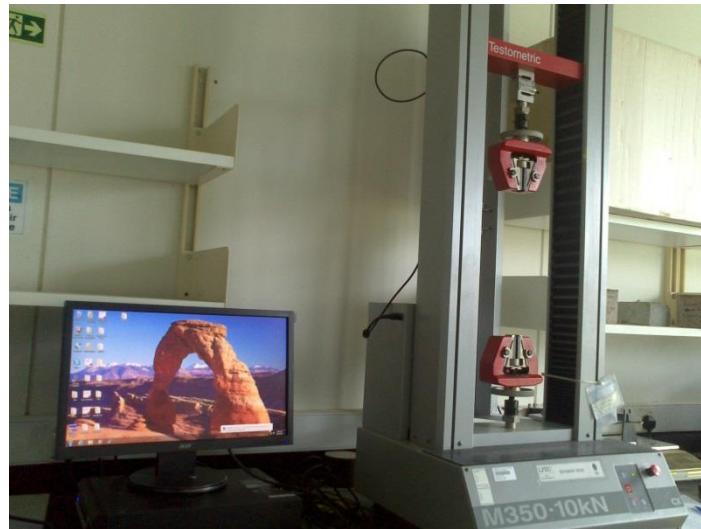
FIGURE 3. 5. Universal Tensile Machine with maximum loading of 10kN.
