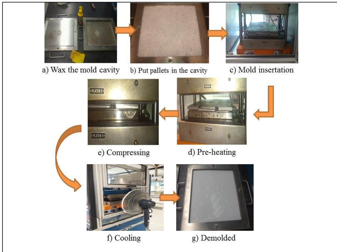
FIGURE 3. 3. Preparation of neat HDPE layer using compression molding.
