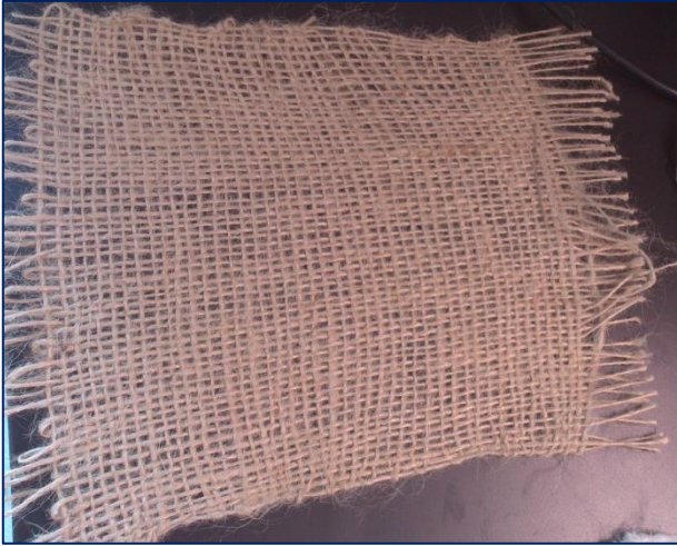
FIGURE 2. 3. Example of plain woven kenaf yarn.
