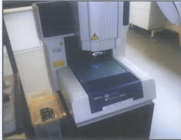
Figure 10: 3D non-contact measurement facility in UTP
