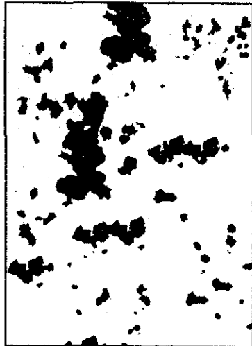
Rust Grade 3-G, 16% Rusted
