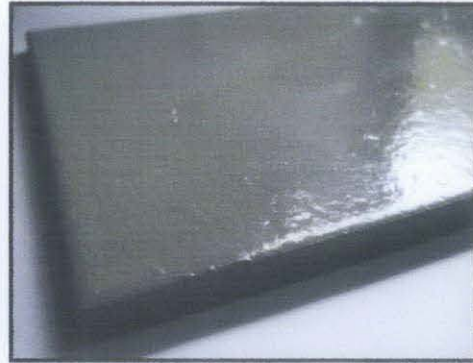
Figure 14: Close-up view on the texture of the plate coated with 2 nd coat
