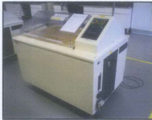
Figure 4: Salt-spray corrosion chamber facility in UTP
