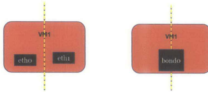
Figure 14: Network Bonding Structure
