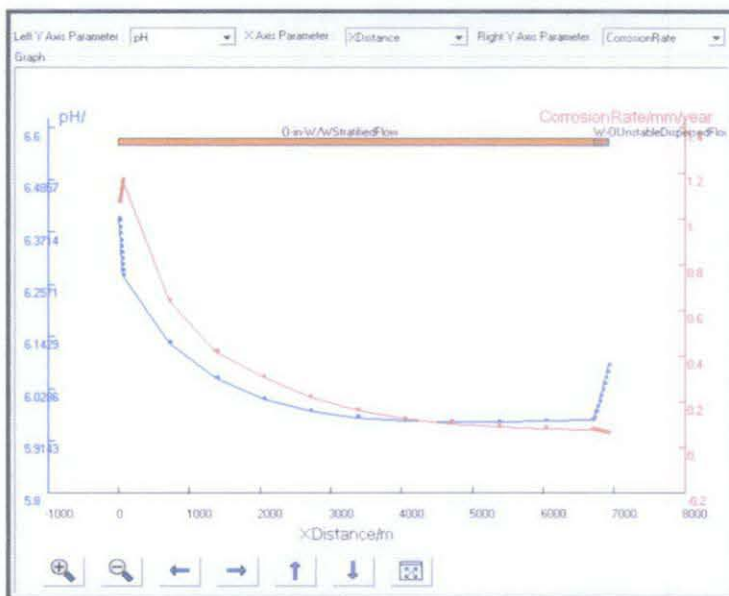
Figure 16: Graph pH vs Corrosion rate along pipeline
