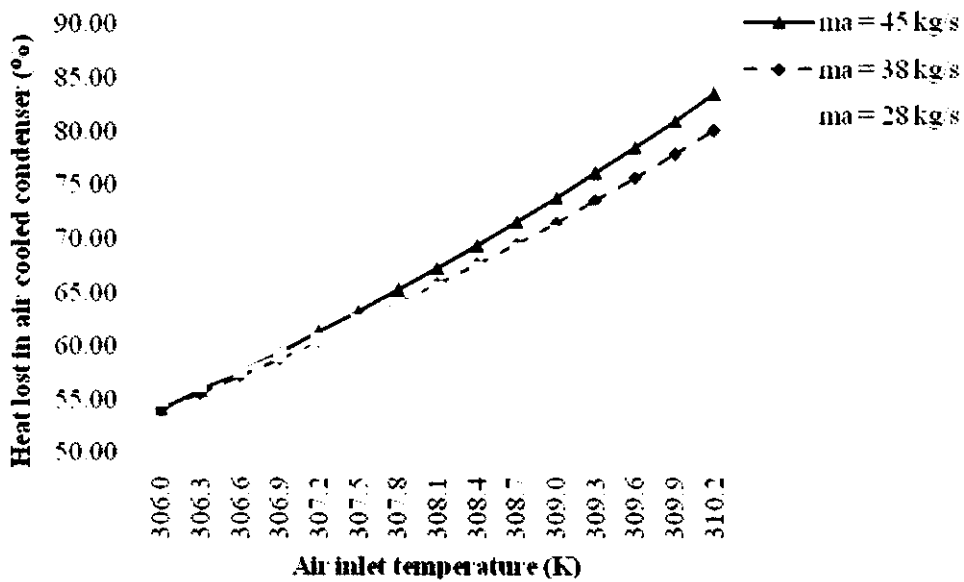
Figure 4.25: Heat energy lost (%) in air cooled condenser against air inlet temperature (K)
