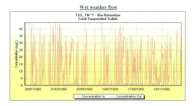
Figure 45: Time-Series Graph of TSS for Sg.Air Putih-after intervention (Wet)
