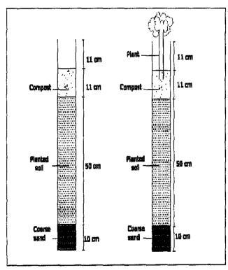
Figure 19: The Design of Bioretention in Laboratory (Variety 1)
