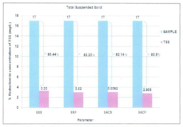
Figure 51: The Percentage Reduction of TSS in Laboratory Model
