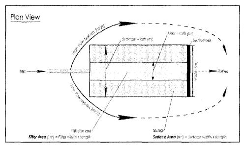
Figure 11: Design of Bioretention in MUSIC Application (plan view)
