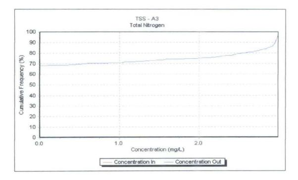
Figure 32: Cumulative Frequency Graph of TN for Sg.Air Putih (Dry)
