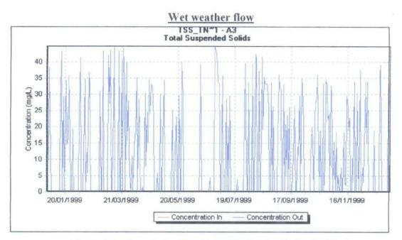
Figure 33: Time-Series Graph of TSS for Sg.Air Putih (Wet)
