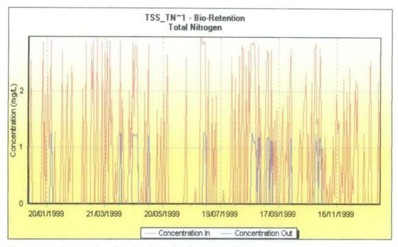
Figure 49: Time-Series Graph of TN for Sg.Air Putih-after intervention (Wet)
