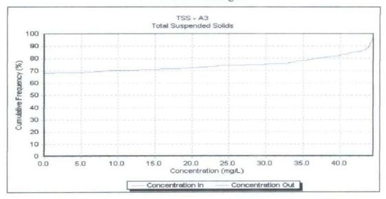
Figure 28: Cumulative Frequency Graph of TSS for Sg.Air Putih (Dry)
