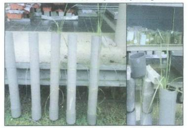
Figure 22: The Physical Model of Bioretention in Laboratory
