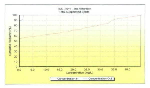
Figure 46: Cumulative Frequency Graph of TSS for Sg.Air Putih -after intervention
