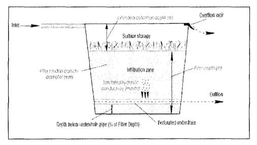
Figure 12: Design of Bioretention in MUSIC Application (longitudinal section)
