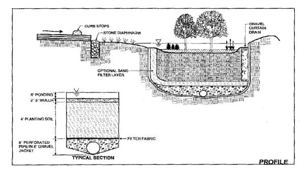
Figure 10: Design of Bioretention (profile view)
