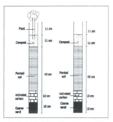
Figure 20: The Design of Bioretention in Laboratory (Variety 2)
