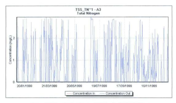
Figure 37: Time-Series Graph of TN for Sg.Air Putih (Wet)
