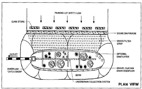
Figure 9: Design of Bioretention (plan view)
